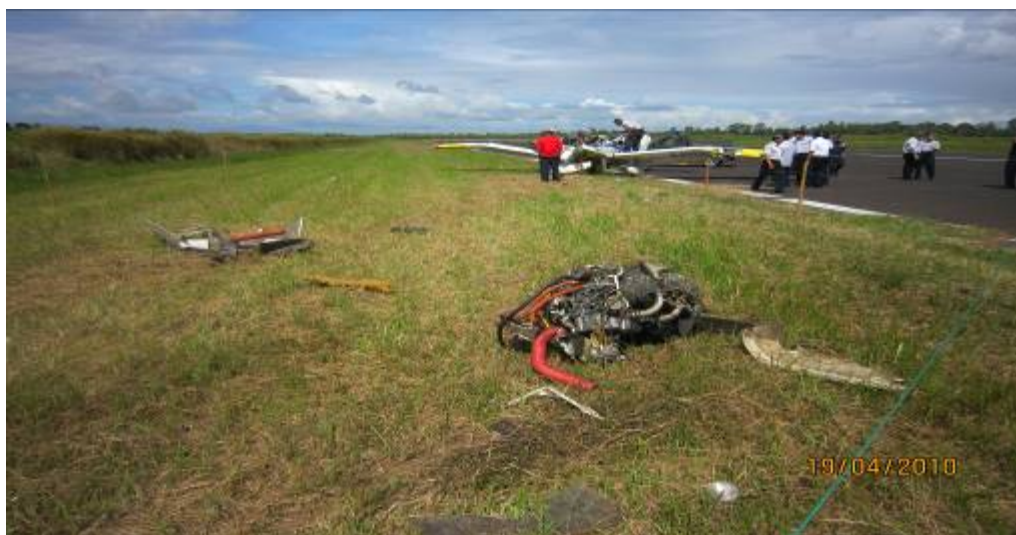
Figure 1: The engine was separated 15 meters from the main wreckage.
