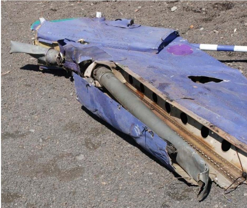
**Figure 8: Twisted tail rotor shaft**
