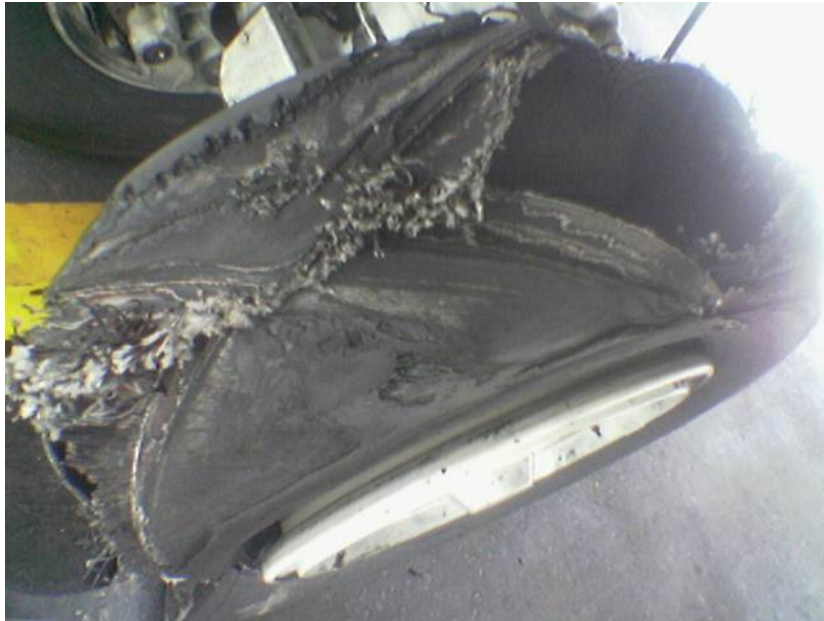
Figure 1: The number-two tire burst.
