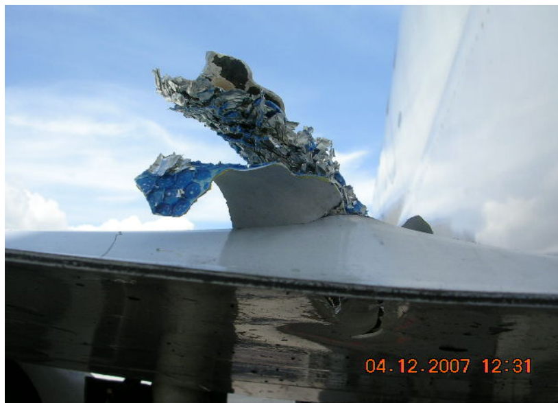
Figure 2: The damage at the aft flap.
