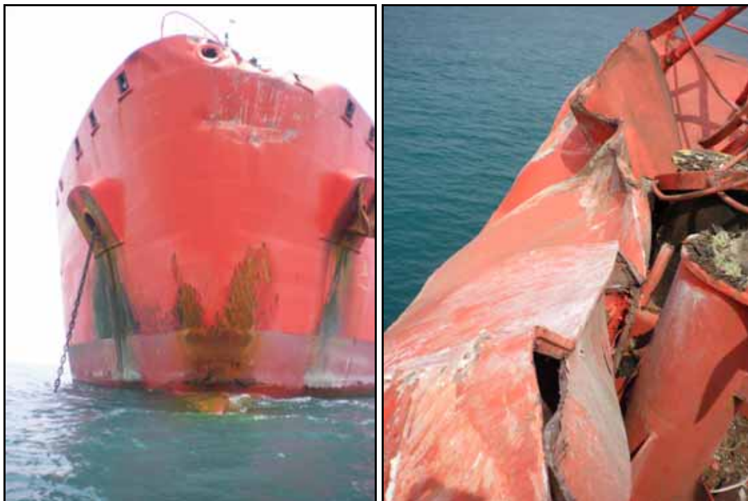
Figurel-9: Collision mark at the bow and ruptured port forecastle's bulwark
