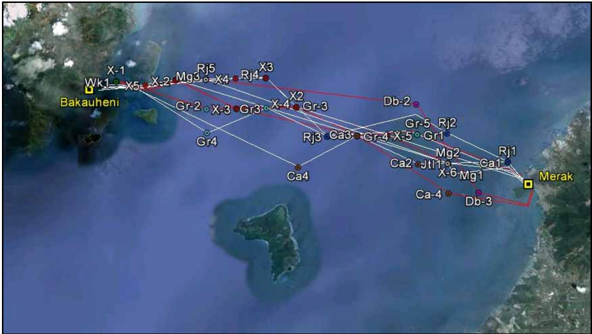
Figure II-1: Merak – Bakauheni ferry manoeuvring pattern based on NTSC survey (red line: ferry to Merak, White Line: ferry to Bakauheni)
