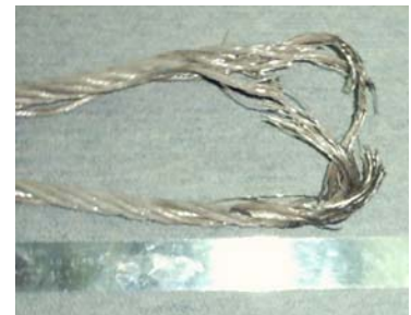
Gambar 13. Sling bogie K9 putus fatigue
